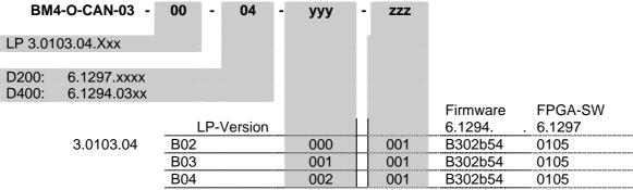
Software-version prototype for firm Battenfeld state of development, it is replaced with official release with firm Battenfeld. (It is replaced afterwards with BM4-O-CAN-03-00-01).
