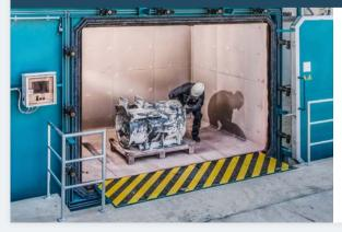
**De-insulation** of motors, generators and transformers by the gentle pyrolysis process.
