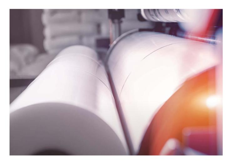
The use of direct drive technology enables the production of very high-quality films, as the lack of gearing means that torque fluctuations can be reduced even at low speeds. With specific functionalities in the converter combined with the servo motors, the cogging torque is almost fully compensated. Using the flexible modular system, machine modules can also be easily connected for further processing.
