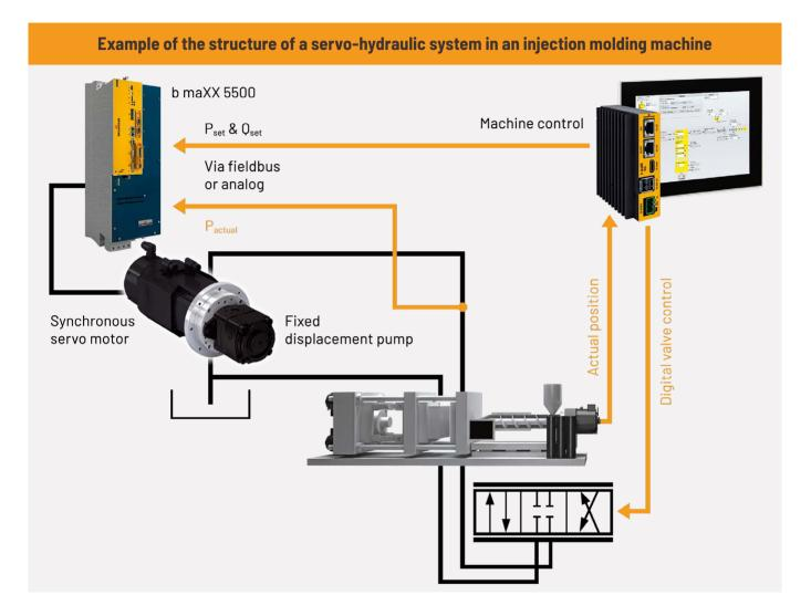
The servo-hydraulic system consists of a servo drive, which drives a synchronous servo motor. This motor drives a fixed displacement pump. The pressure and volume flow set values (Pset and Qset) are sent from the control unit to the servo drive. Pressure and flow rate are controlled on the servo drive by adjusting the speed. As in the conventional hydraulic systems with standard motors, the actual positions are read out via the machine control unit.
