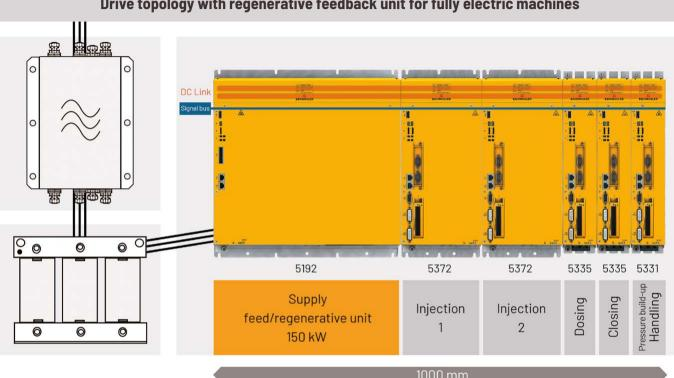
Drive topology with regenerative feedback unit for fully electric machines
