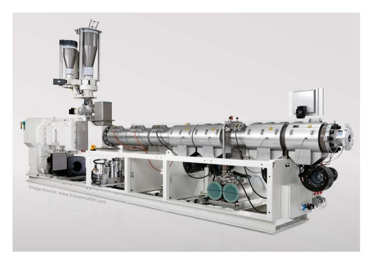
Baumüller offers energy-efficient direct drive technology for extrusion machines. With this technology you can minimize drive losses, reduce background noise during operation and increase the reliability of the machines. At the same time, the lack of gearing means a smaller size for the machines, which can be designed more compactly. For special ambient conditions, such as powder processing or production in high humidity regions, water-cooled motors can be used.
