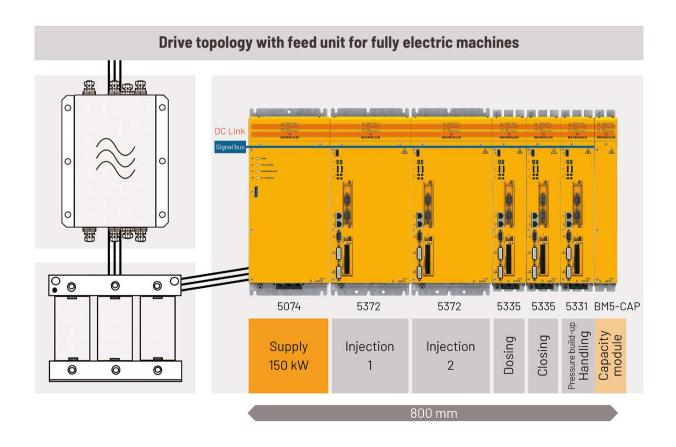
In addition to supplying power to the power modules, the use of a regenerative feed unit also enables the sinusoidal feedback of excess braking energy into the power supply system. This regenerative system thereby makes an additional contribution to reducing energy consumption.
