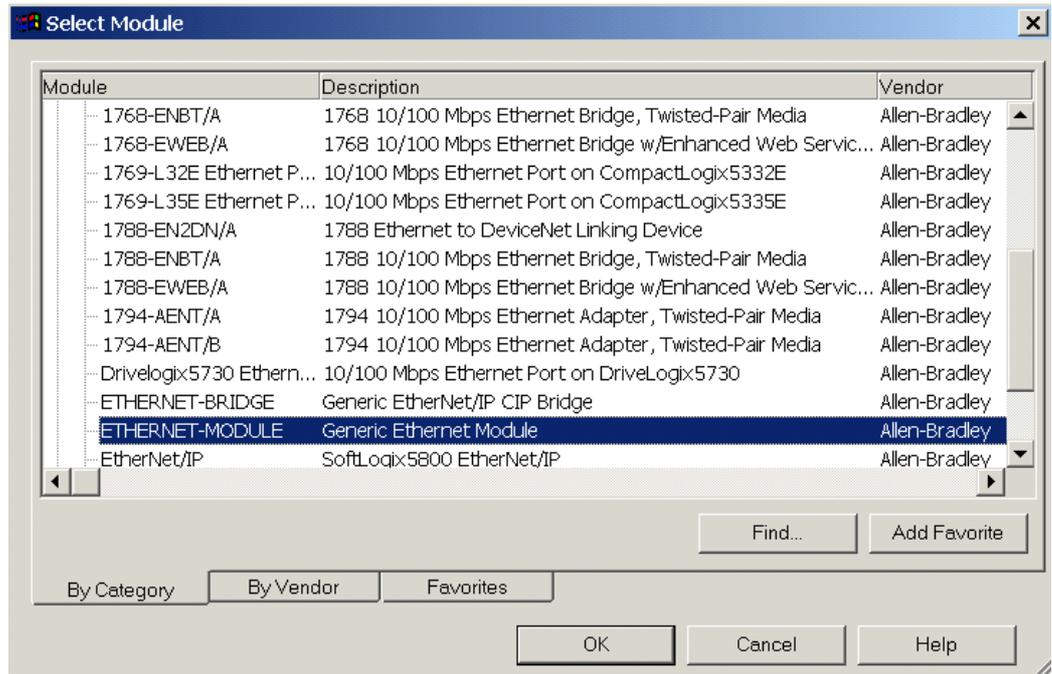
Figure 6: Selecting Generic EtherNet Module
