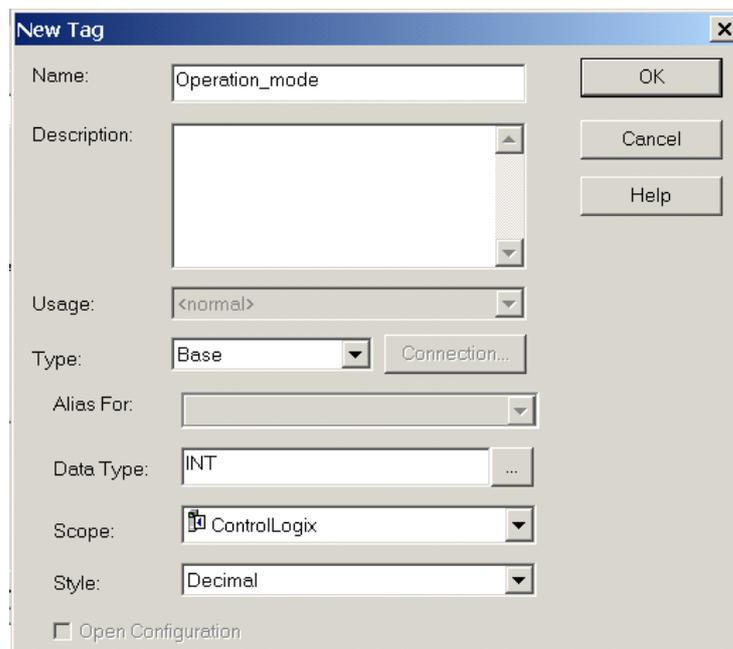
The screenshot shows the 'New Tag' dialog box. The 'Name' is 'Operation\_mode'. The 'Description' is empty. The 'Usage' is '<normal>'. The 'Type' is 'Base'. The 'Alias For' is empty. The 'Data Type' is 'INT'. The 'Scope' is 'ControlLogix'. The 'Style' is 'Decimal'. There is an 'Open Configuration' checkbox. At the bottom right are buttons for 'OK', 'Cancel', and 'Help'.
