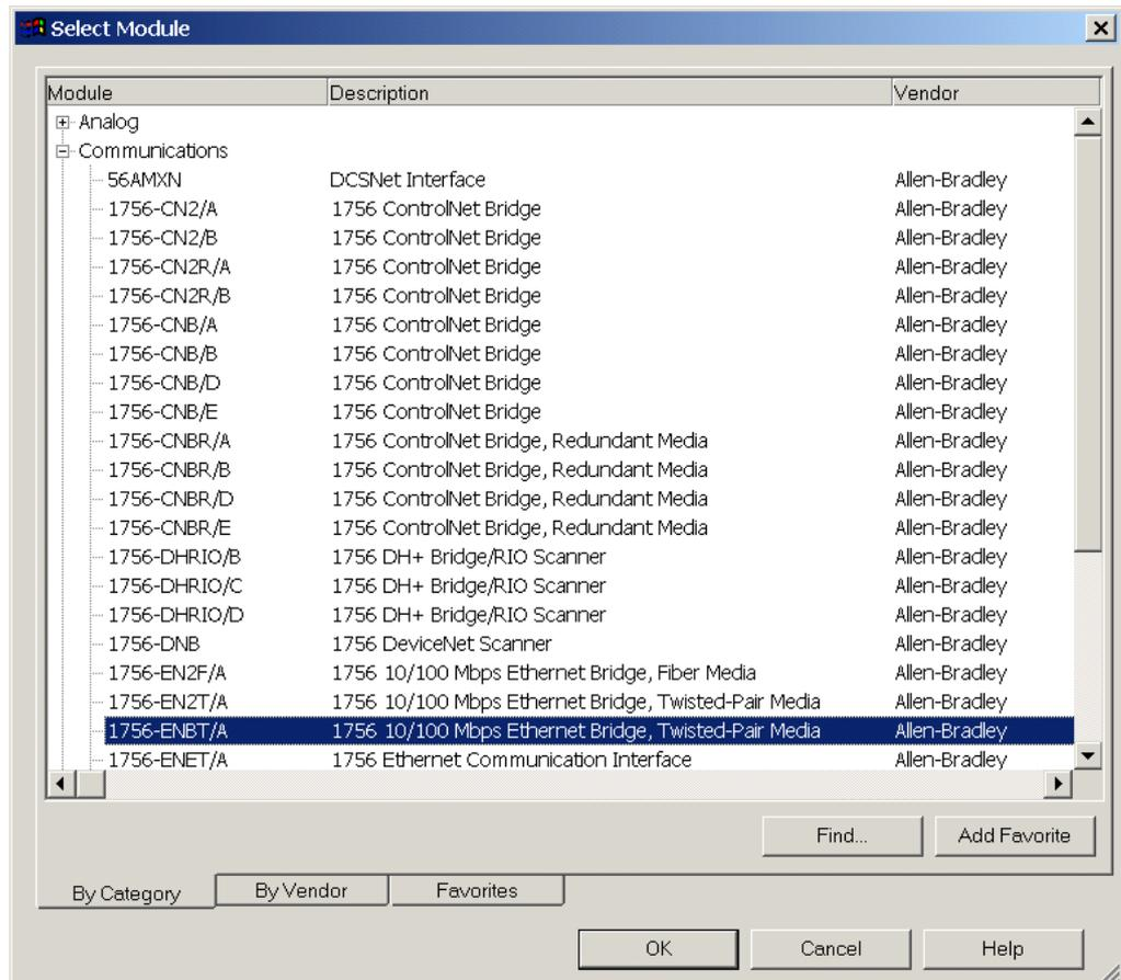
Figure 4: Selecting the EtherNet Bridge
