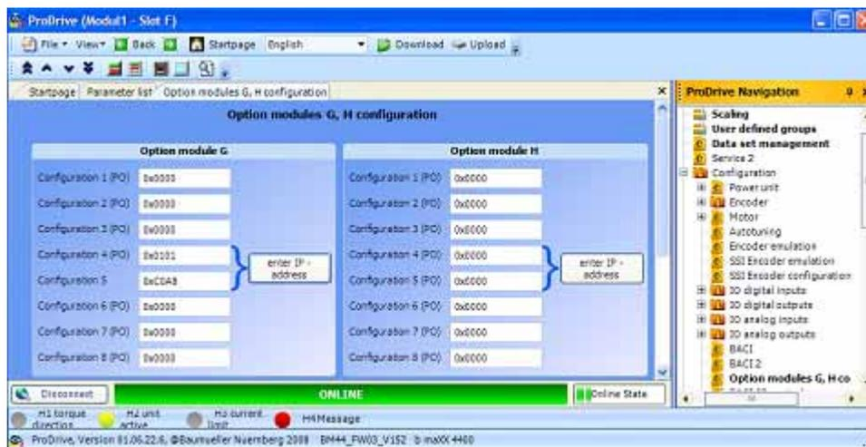
Figure 2: IP addressing by controller
