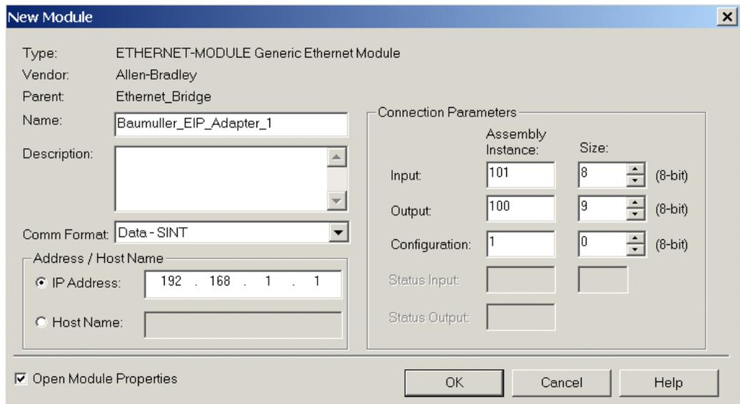
Figure 7: New Module configuration
